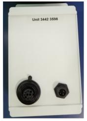
services. A self-contained IP65 sealed dedicated wireless interface module (WIM) with an integrated SIM and internal antenna is co-located with and connected to a detector and requires only access to the usual 24V d.c. supply to operate. In effect, the WIM replaces the wired link from the detector to the O.T.U with a link that uses mobile data.
